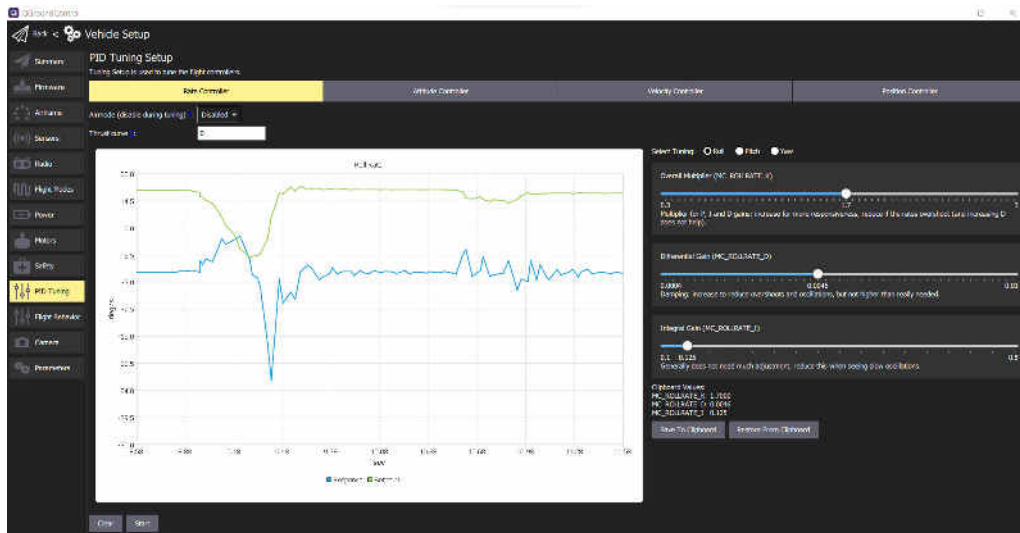
Figure 3.23: PID Tuning Interface of QGroundControl
