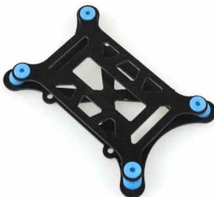
Figure 3.24: Vibration Absorber Base for Pixhawk (Image source: (6))
