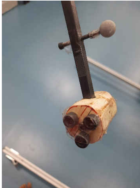
Figure 4.28: Bolts to adjust the mass of the pendulum
