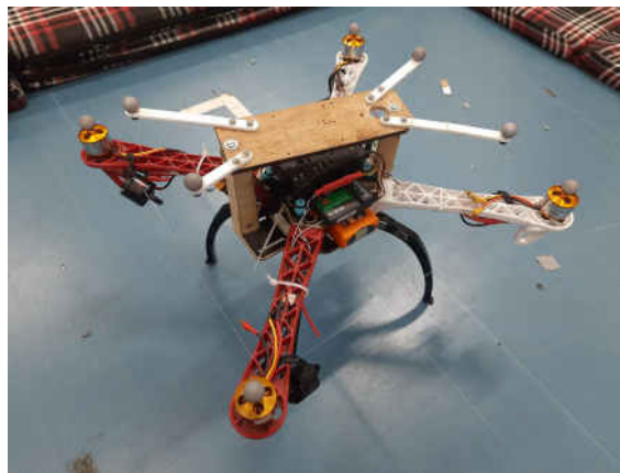
Figure 3.34: Alignment of the Pixhawk Body Frame with Vicon World Frame
