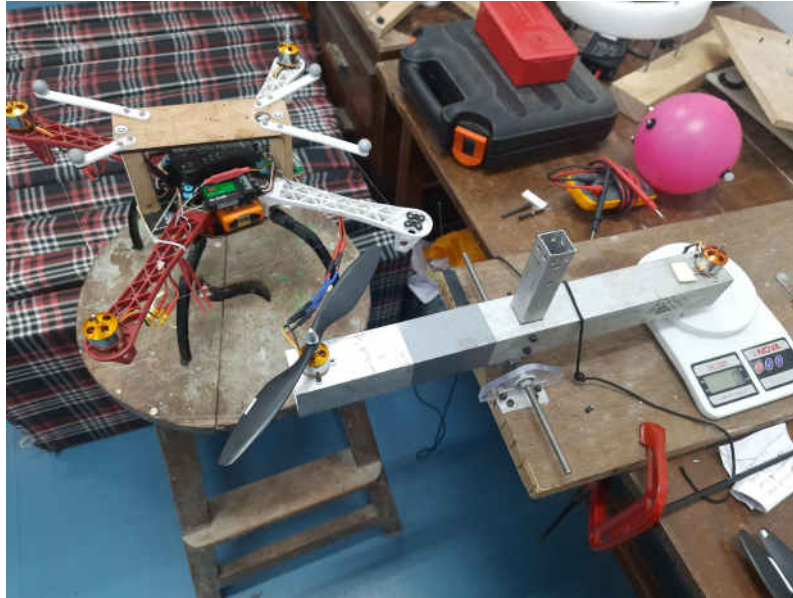
Figure 3.15: UAV on Thrust Measurement Setup
