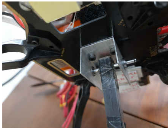
Figure 4.29: Pendulum Attachment to the UAV
