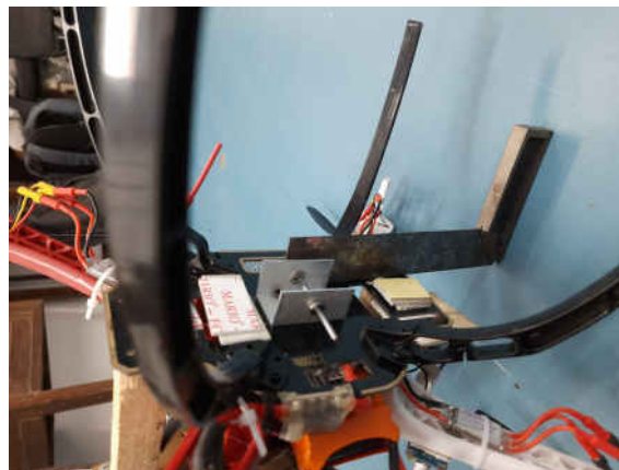
Figure 3.36: Calibrating Pixhawk Sensors using Right Angle Protractor
